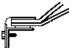
**Rounded Rail:** Again, the domes have to be small enough to fit inside the rail. Sometimes, these rails are really wide and the dome may not be able to fit under the rail as pictured here, but have to fit inside another groove on the frame. Best to get actual dome measurement.
