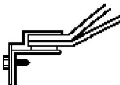
**Notched Rail:** The domes have to set inside the “second step” of the rail when the rail is notched. If you measure that upper notch as a rail measurement it will be a good measurement in most cases as long as the rail isn't wider than 1 ¾”.
