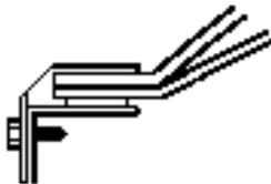
**Beveled Rail:** From the picture you can see the domes have to be small enough to miss the bevel of the rail. If the rail isn't very wide, usually you can measure from the bevel to the bevel, but again—when in doubt—take the rail off and measure the actual domes.
